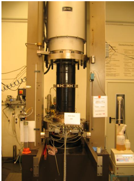
Figure 1. Testing equipment and salt samples of large sizes tested in laboratories at GRS for research on damage behavior and impacts during coupled THM processes, WP3, THERESA project.
