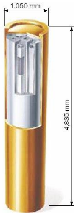
Figure 2. The full scale Canister Retrieval Test (CRT) at SKB's Äspö hard Rock Laboratory (HRL), Sweden, used for WP4, THERESA project. a) Illustration of the experimental set-up and the location in the TASS tunnel; b) The deposition hole after installation of the mats during installation of the bottom block; c) Installation of the canister; and d) KBS-3 canister parameters.
