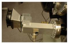
the waveguide components to be made. The POLYDRY 'pilot' microwave drying system was successfully built, assembled and initial vacuum Tests were carried out before shipping to Sonderborg Plast where the waveguides, magnetrons, power supply was fitted and control system integrated together. The waveguides were fine tuned and initial checks performed before validation trials phase.
