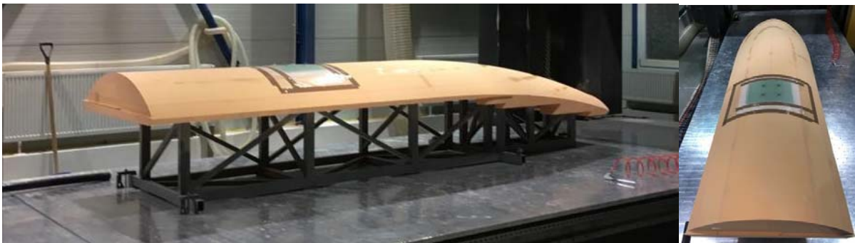
Fig. 61: Fairing mold after milling (left) and GFK lay-up of access hole (right)
