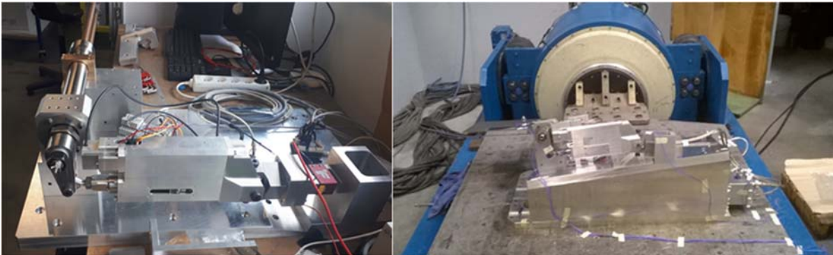
Fig. 11: Test bench for functional tests of the actuator (left) mounted on vibration table (right)
