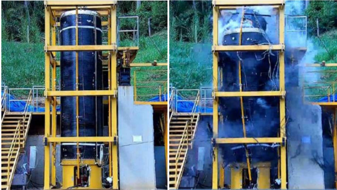
Fig. 59: S50 motor case burst test at AviBras
