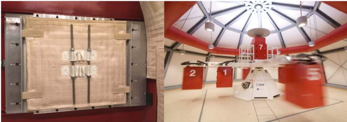
Fig. 17: Customized internal thermal protection system fixation with Velcro (left) and testing under acceleration (right)
