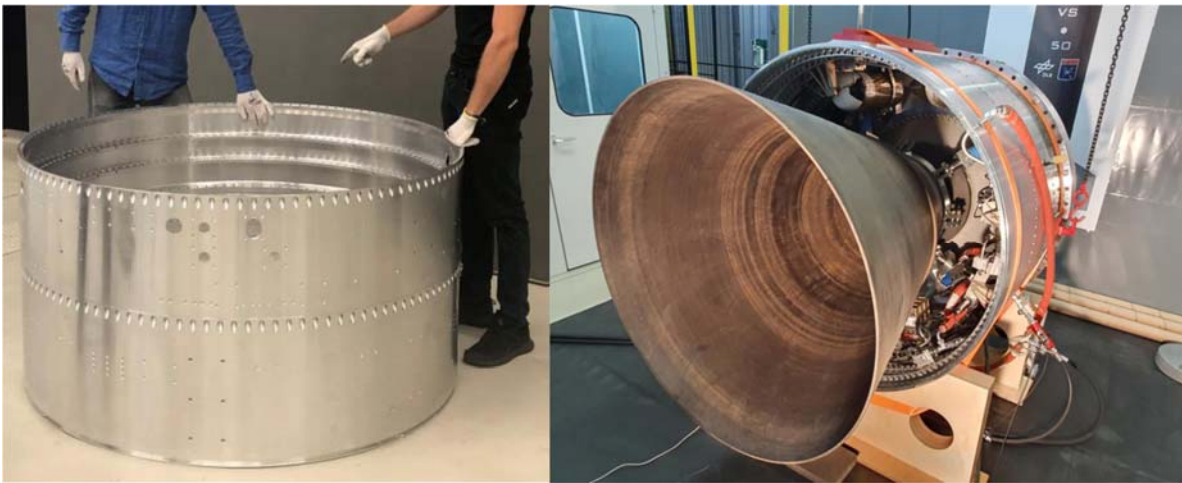
Fig. 60: Tailcan flight hardware (left) and integrated TVA (right)
