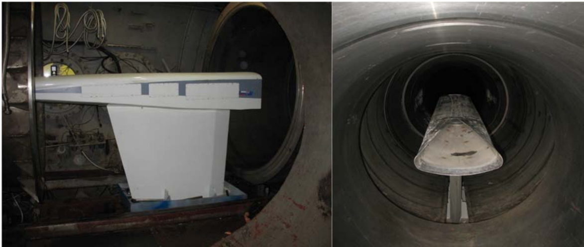
Fig. 52: Low thermal heat inertia scramjet module installation in the CIAM free-jet facility.
