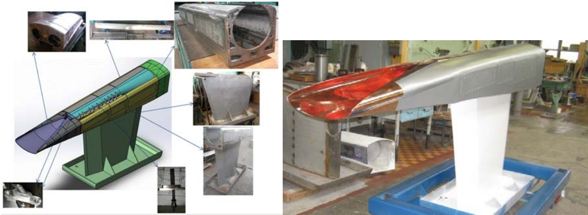
Fig. 51: The full-scale EFTV scramjet module with low (left) and high thermal heat inertia (right).
