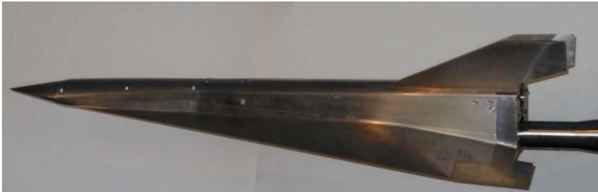
Fig. 21. The model of the EFTV Glider Option mounted on a sting.
