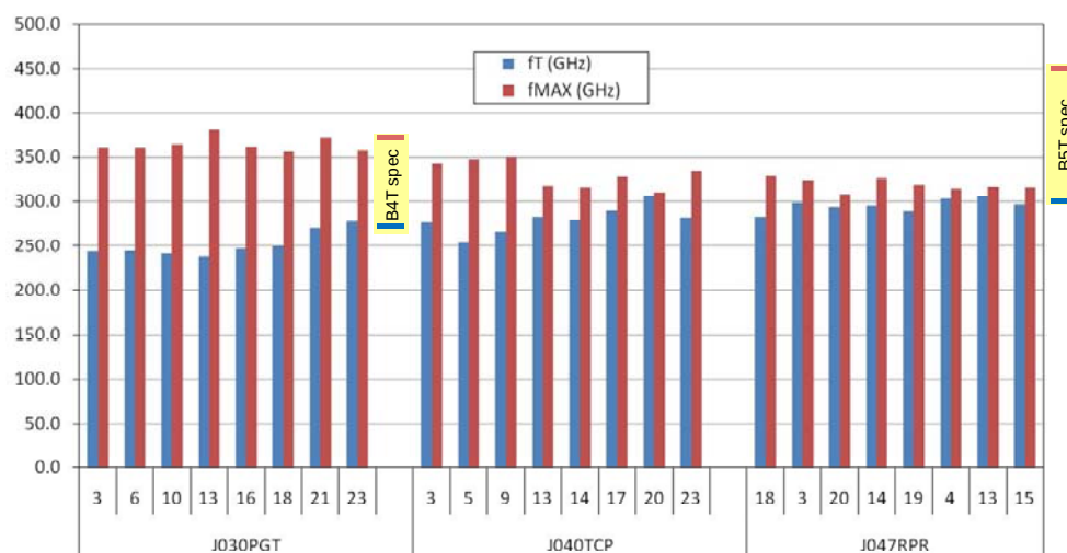
Figure 6: f_T , f_{MAX} performances measured on 24 splits done on vertical profile from 3 different lots with B4T design rules (wafer average values for 0.11 \times 4.9 \mu m^2 transistors)
