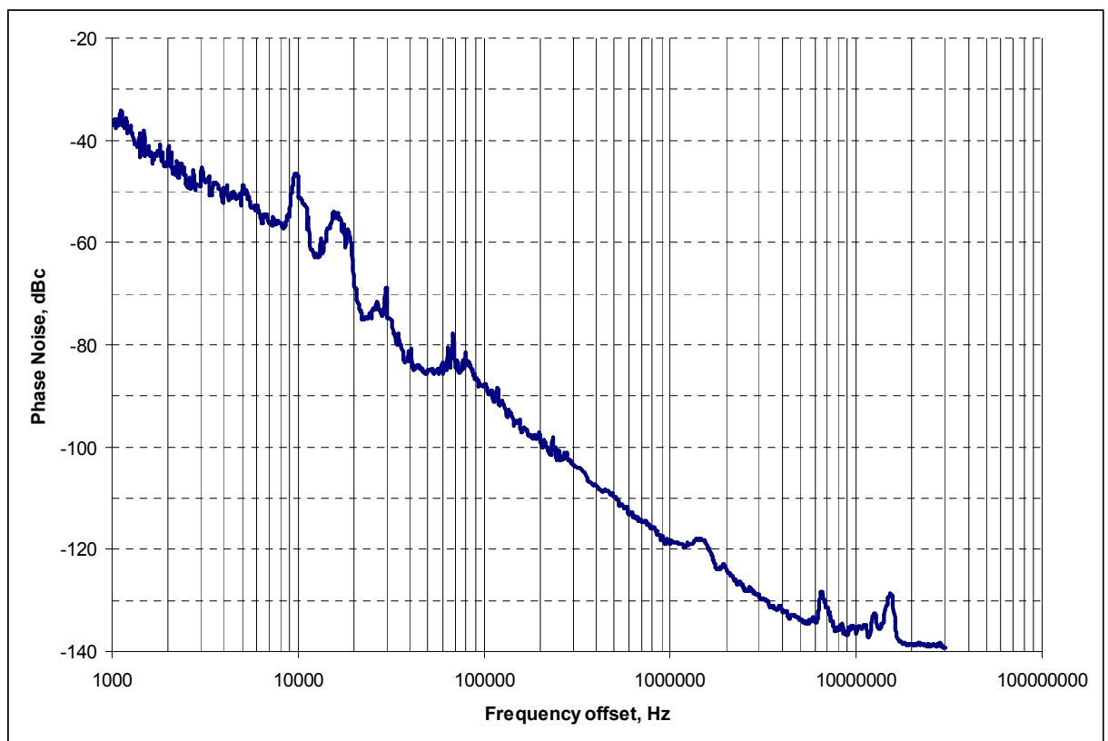
Figure 54: Phase Noise of the VCO, measured at the divider output
