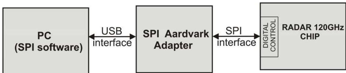
Figure 39. PC, Aardvark Adapter and Radar 120 GHz chip.
