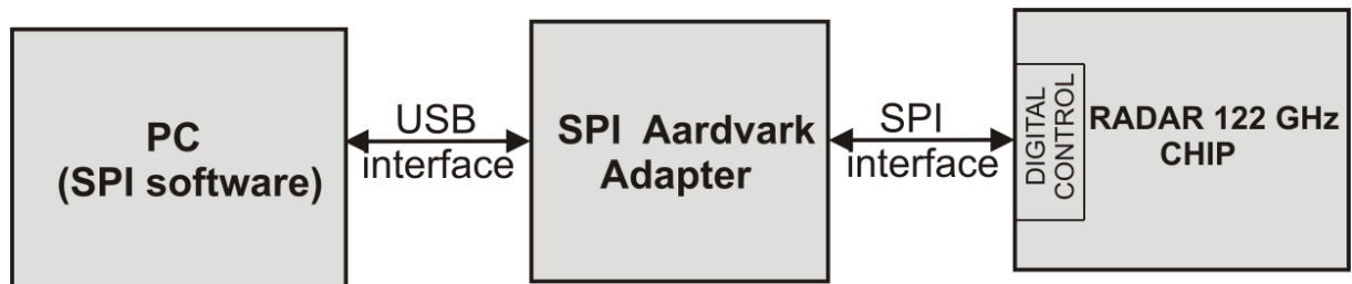
Figure 9 PC, Aardvark Adapter and Radar 122 GHz chip
