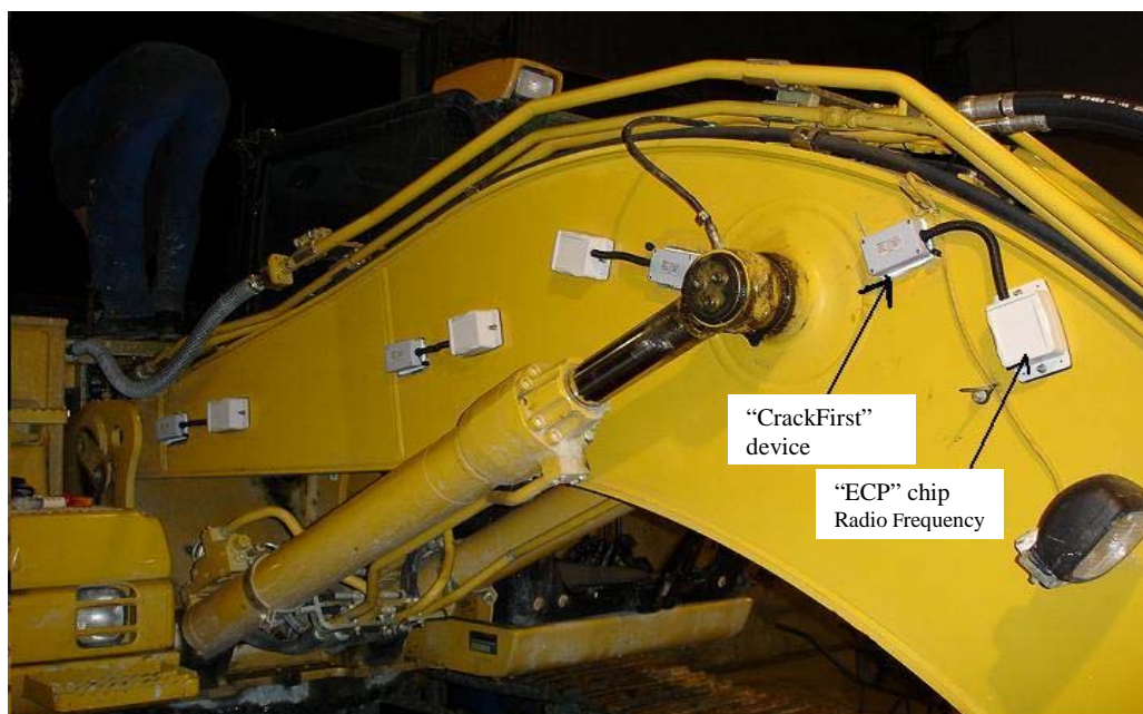
FIGURE 6: BOOM EXCAVATOR EQUIPPED WITH FOUR COMPLETE FATIGUE DEVICES (FEB-07)
