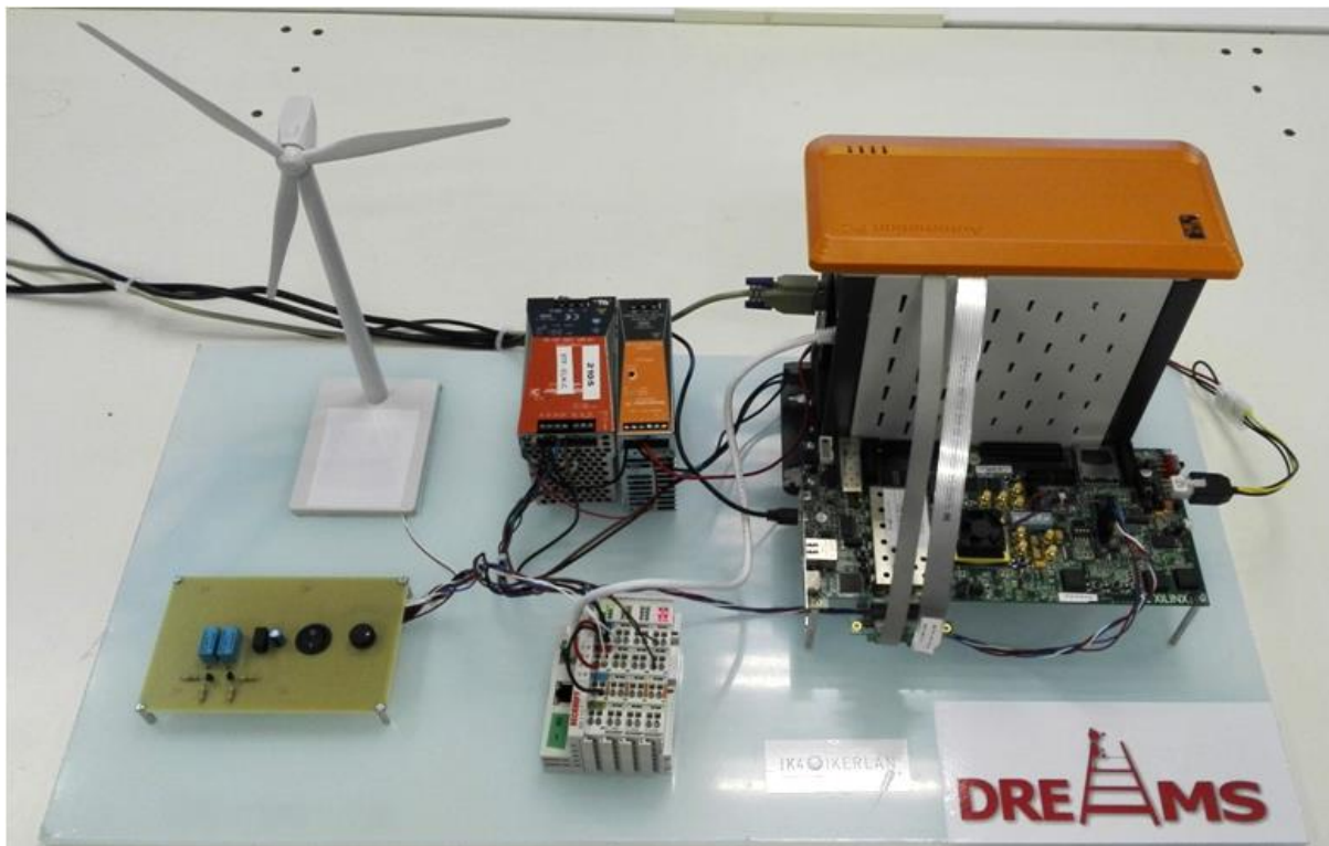
Figure 14: DREAMS wind-power demonstrator.
