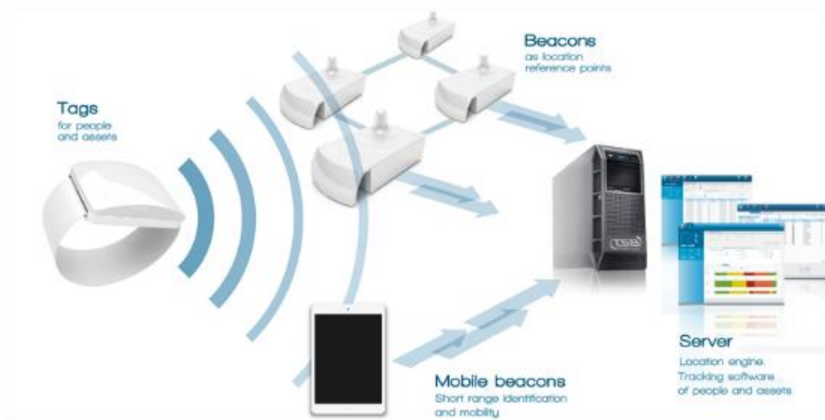
Figure 18 MYSPHERA RTLS working diagram
