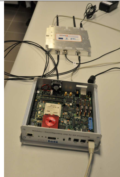
Figure 3-4: Testbed 1 simplified transmitter/receive chain with RF and PHY integrated
