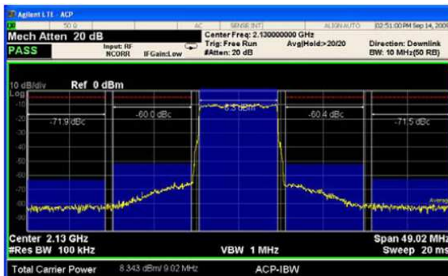
Figure 2.24: ACLR in commercial HPA (+10dBm over 10MHz)
