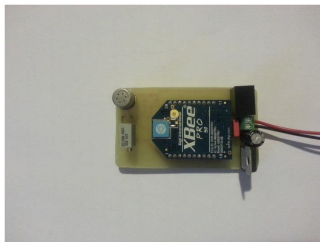
Figure 5 The gas sensor coupled with a Xbee device.
