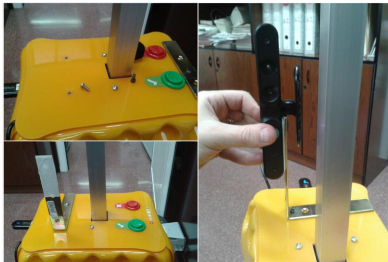
Figure 7. The RGBD camera cannot be placed directly on the neck as in previous versions. Instead, it must be mounted using a L-shaped mounting bracket.
