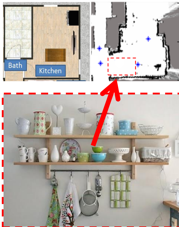
Figure 12. Furniture such as shelves above 1.20 m. are outside of the field of view of the RGB-D camera.
