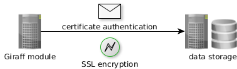
Figure 19. Secure communication channel
