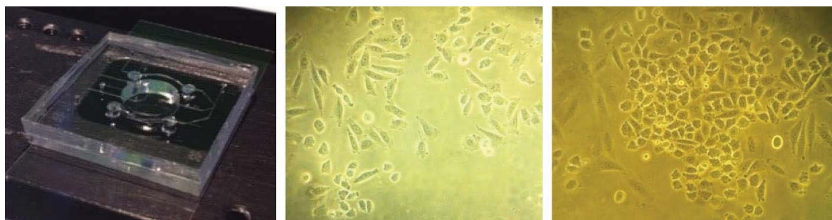
Figure 38: CHO cells were cultured during 5 days inside a PDMS, where cells differentiated and spread normally.
