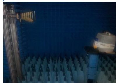
(c) EME-SPY 140 with body liquid at +20^\circ incidence (vertical polarization)
