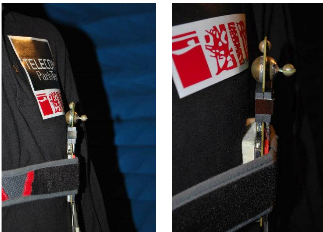
Figure 58 : Sensor/phantom spacing: ~ 0, 10 and 20 mm (not shown here).
