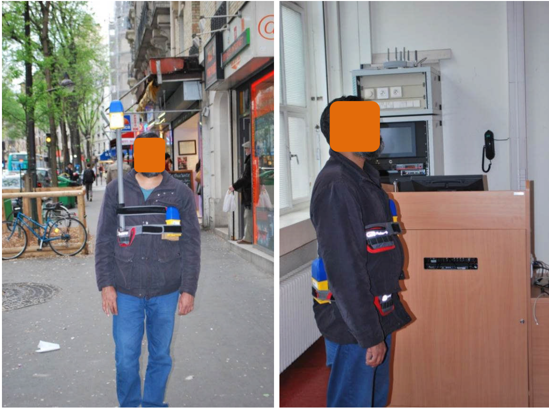
Figure 109 : Measurement configurations with two dosimeters (used in both outdoor and indoor environments). Left: on the chest and “isolated”, right: on the chest and on the back.
