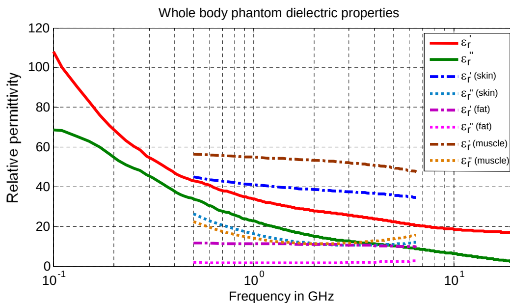
Figure 55 : Whole body phantom (“Kevin”) dielectric properties (from [17]).
