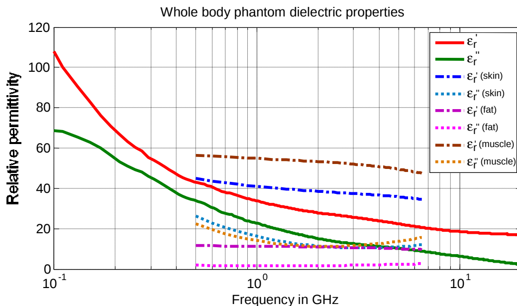
Figure 49 : Whole body phantom (“Kevin”) dielectric properties (from [17]).
