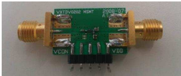
Figure 16 : Photograph of the VMMK-2303 evaluation board
