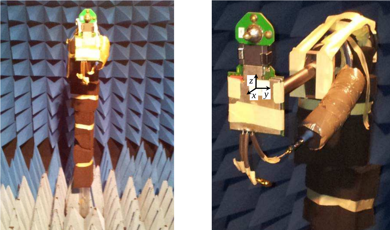
Figure 37 : Experimental setup for the measurement of the isolated sensor in anechoic chamber.
