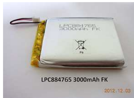
Figure 35 : Flat battery identified for the LEXNET dosimeter
