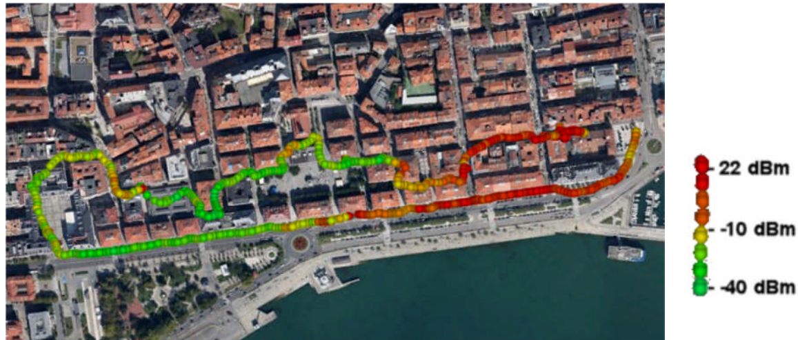
Figure 6: Example of 3G Tx measurements in Santander downtown area
