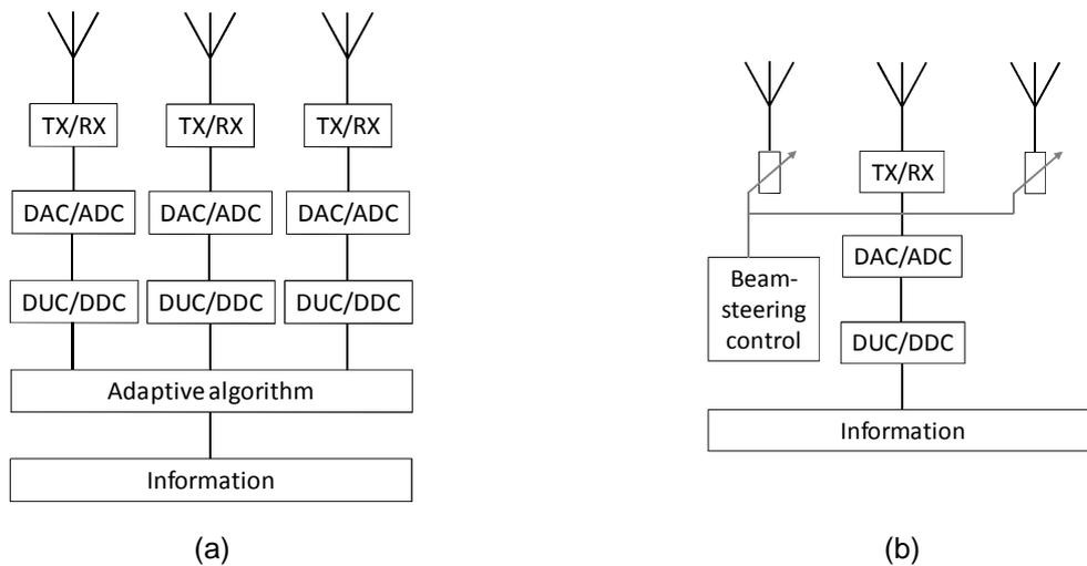
**Figure 13** Block diagram of a conventional digital beam-forming transmitter/receiver system (a) and the architecture based on electronically reconfigurable parasitic array antenna (b).
