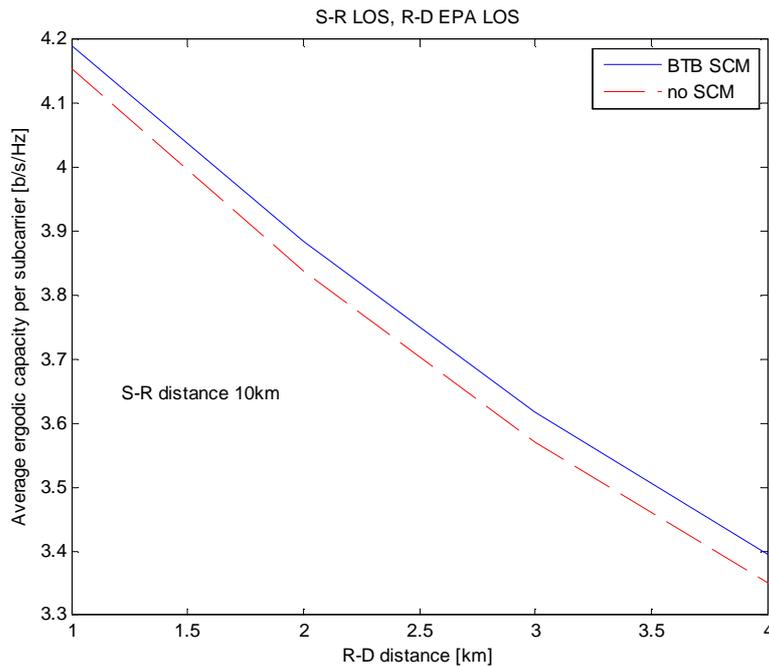
**Figure 50 Average ergodic capacity per subcarrier for OFDM DF systems with BTB SCM and no SCM (S-R LOS, R-D EPA LOS scenario)**
