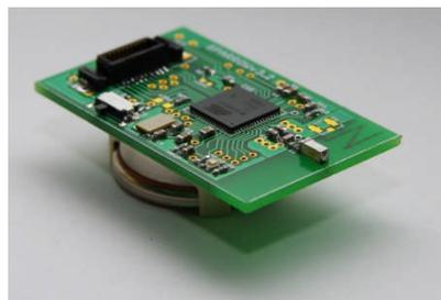
**Figure 44** our test-bed consists of these Sparrow v3 nodes
