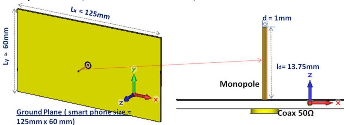
Figure 57 Monopole antenna configuration.
