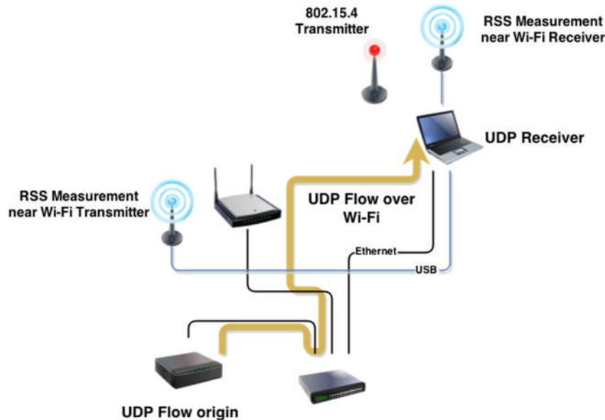
**Figure 45: Testbed arrangement for RSS (Received Signal Strength) measurements of Wi-Fi traffic**
