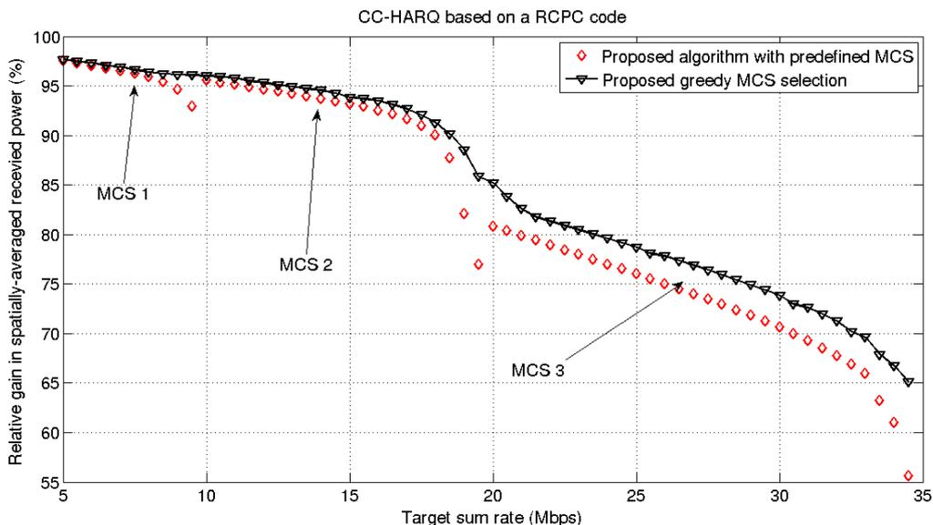
**Figure 56 Spatially-averaged received power (KPI) gain vs. Sum target rate for the proposed algorithms when CC-HARQ is implemented**
