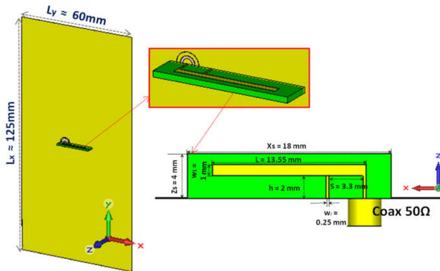
Figure 58 IFA Antenna configuration
