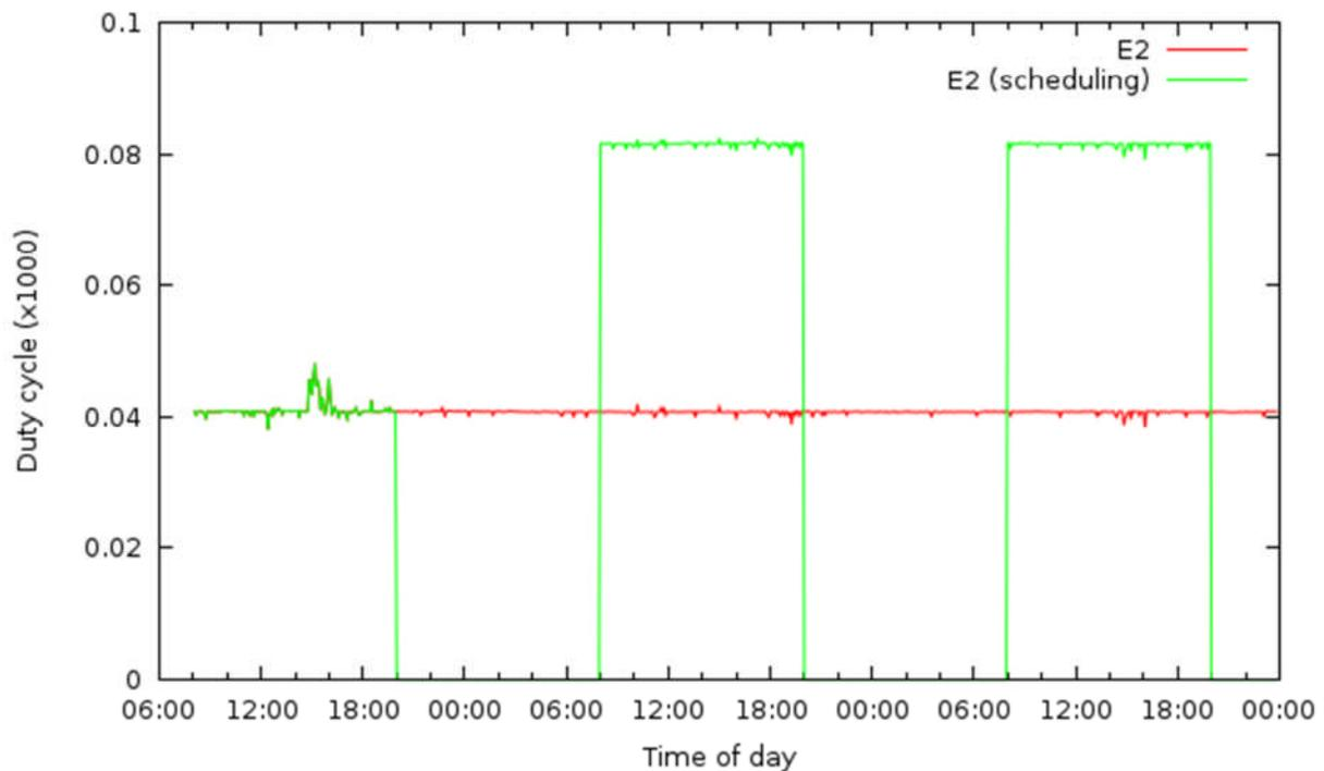
Figure 49 - Transmitter duty cycle with static scheduling
