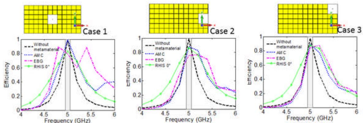
Figure 69 Efficiency. Case 1: antenna at centre. Case 2: antenna at middle of the edge. Case 3: Antenna on the corner
