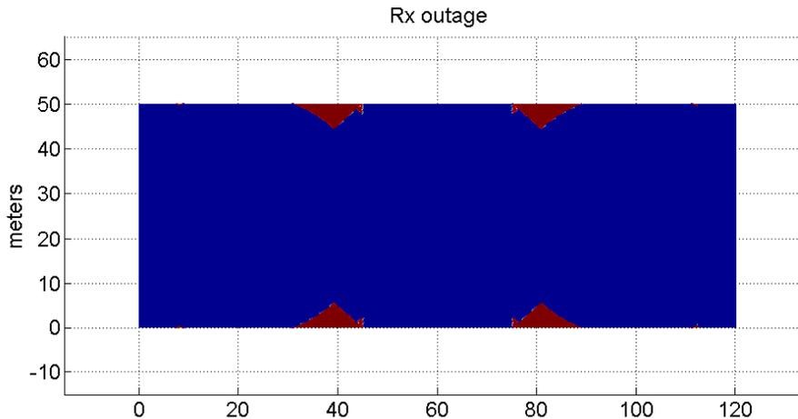
**Figure 40** Outage map with all APs running in SISO idle mode (red area, 2.4GHz)
