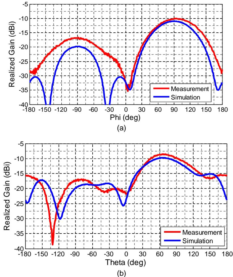
**Figure 20** Measured and simulated directivity radiation pattern (simulation frequency 868 MHz, measurement frequency 881) of the three-element computed on the (a) H- and (b) E-plane.
