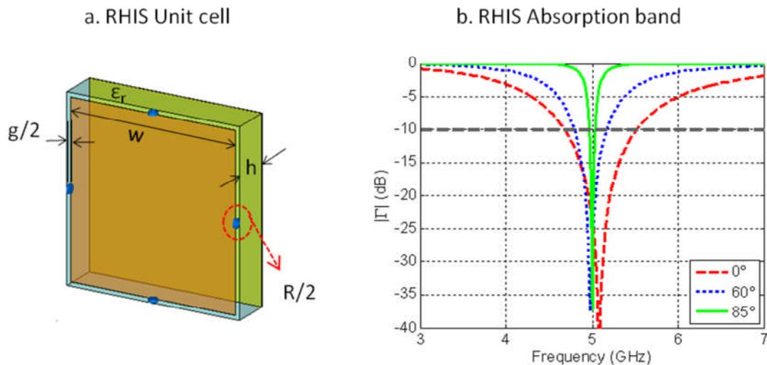
Figure 61. RHIS configuration and Absorption bandwidth
