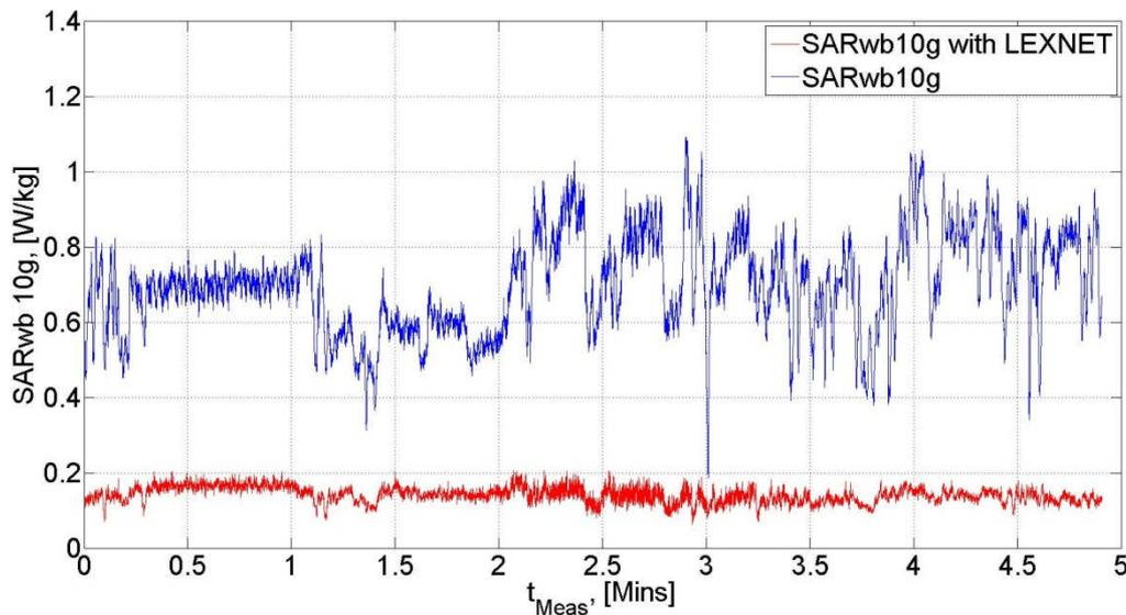
Figure 12: SARwb10g calculations with and without LEXNET.
