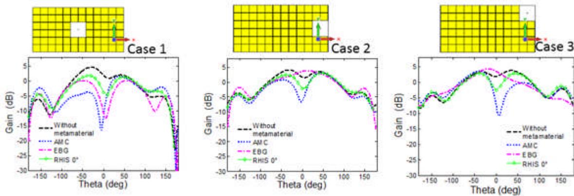
Figure 71 Gain Radiation pattern. Plane  $\phi = 0^\circ$ . Case 1: antenna at centre. Case 2: antenna at middle of the edge. Case 3: antenna on the corner
