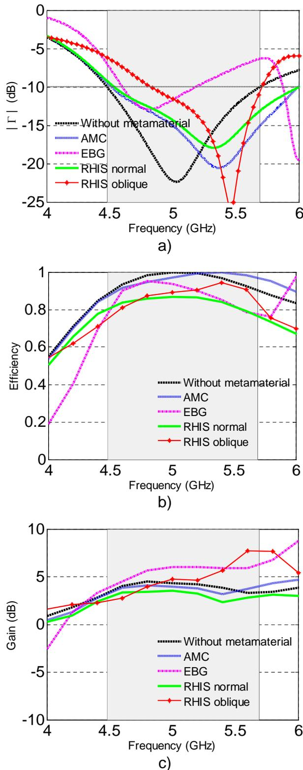
Figure 5 QoS KPI Monopole Antenna a) Antenna matching b) Total efficiency c) Gain
