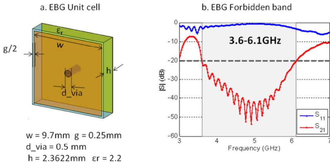
Figure 60. EBG structure and bandwidth
