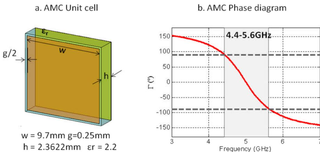
Figure 59. AMC Unit cell and Phase diagram
