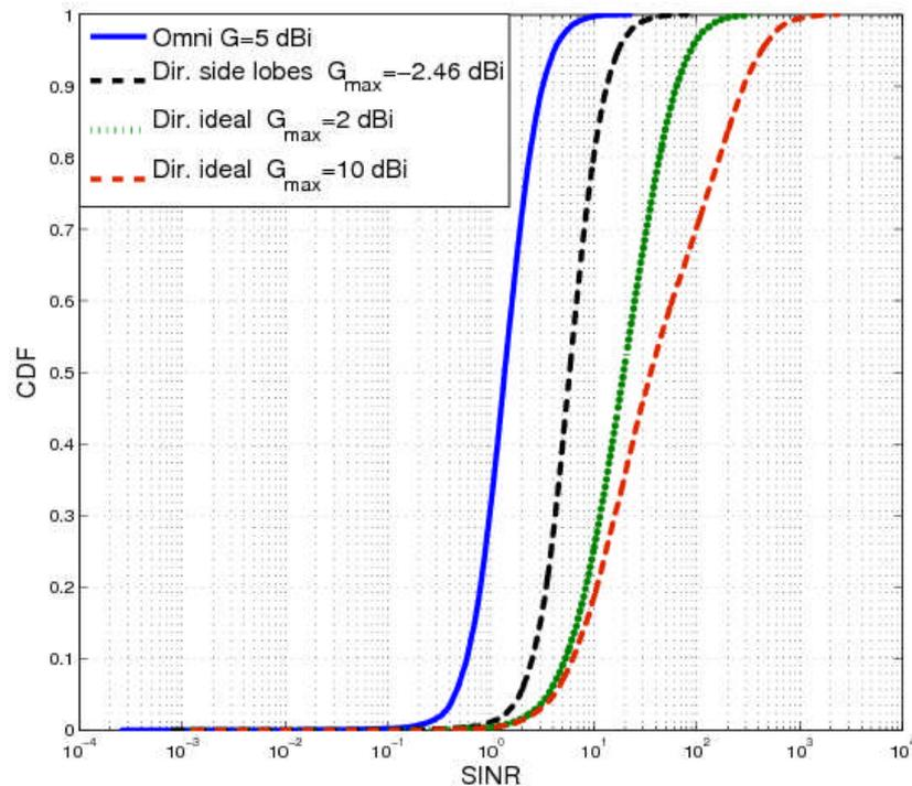
**Figure 22 Cumulative distribution functions of the average uplink SINR at SCs with respect to different antenna patterns and a REB equals to 3 dB.**
