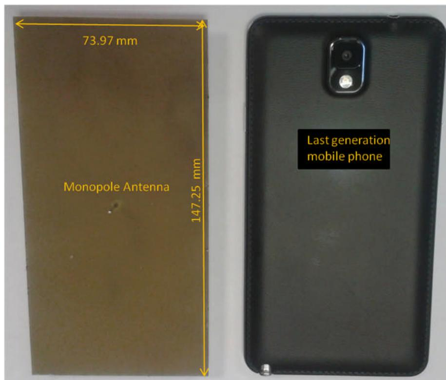
Figure 74 Monopole antenna without metamaterials
