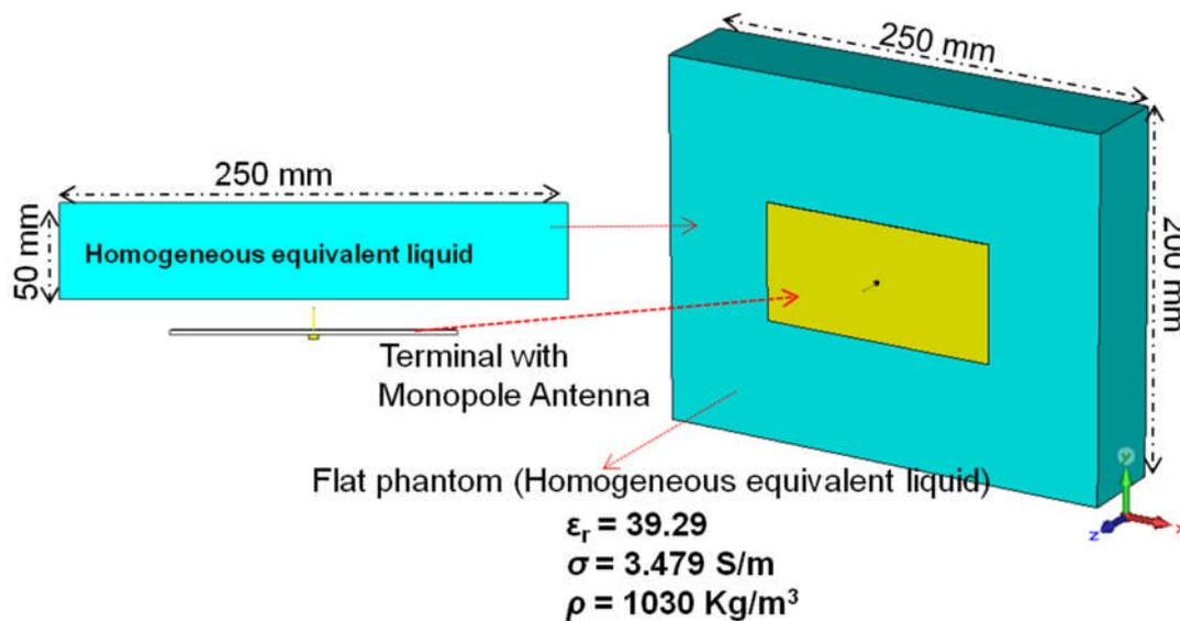
Figure 4 Simplified model for exposure simulation
