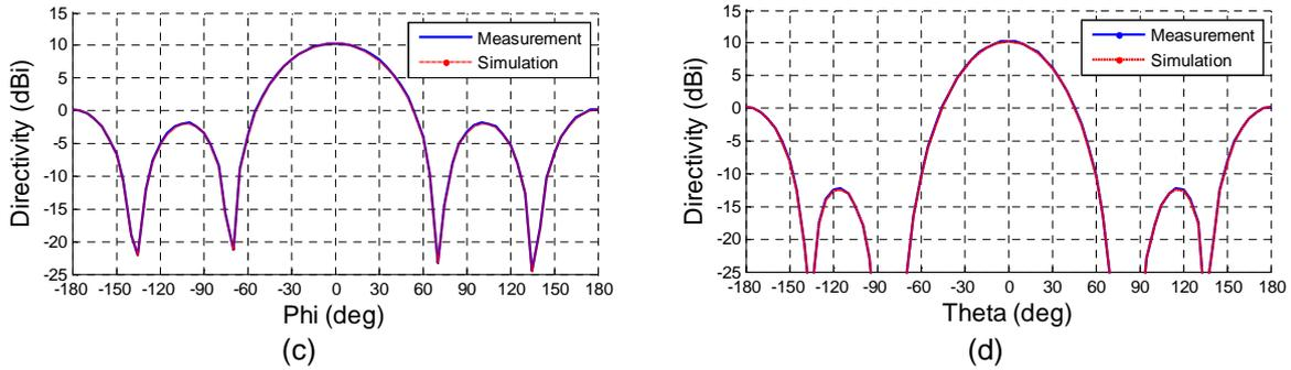
**Figure 16 Directivity pattern (Co-polar and Cx-polar components) of the three-element array calculated at 868 MHz. 3D (a) theoretical and (b) simulated results. (c) H- and (d) E-plane.**
