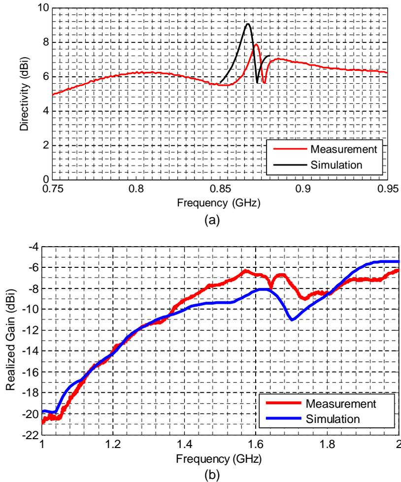
**Figure 18 Measured and simulated maximum directivity as function of the frequency in the case of (a) three-element and (b) four-element array**
