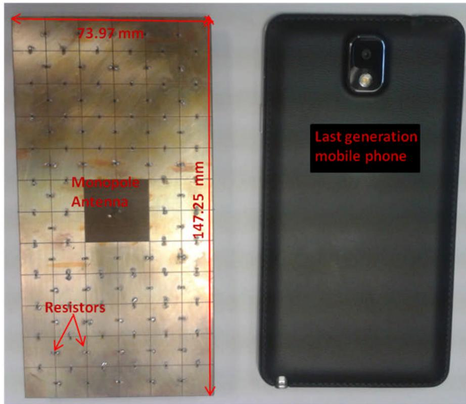
Figure 75 Monopole antenna with RHIS structure
