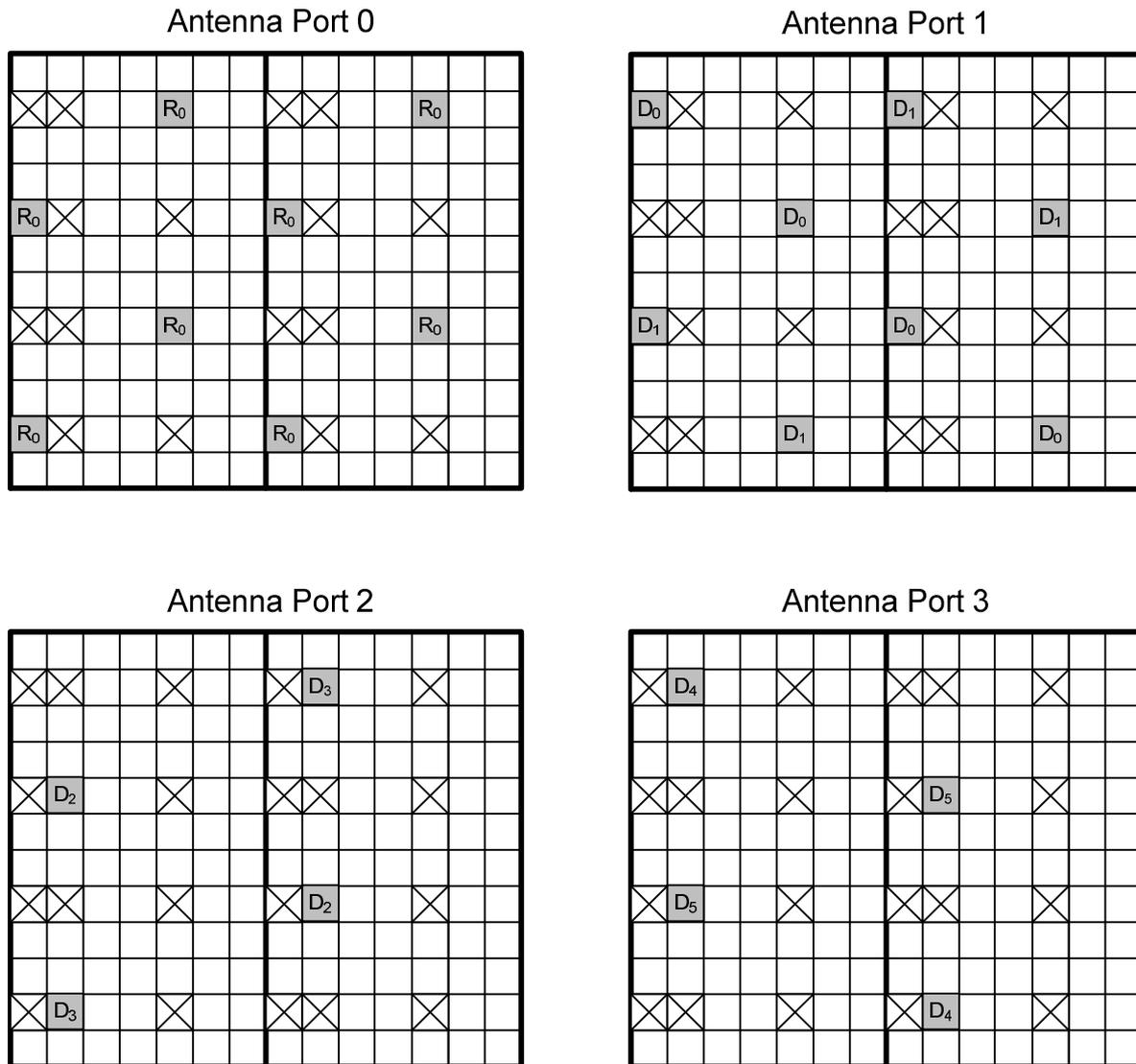
Figure 42 DMRS configured on 3 CRS antenna ports in the 4 CRS ports case in LTE RBs
