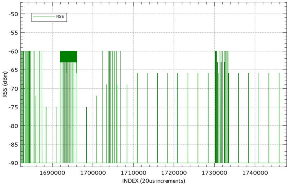
Figure 47 The same sequence with a higher resolution timescale show individual Wi-Fi packets failing and the router backing off, slowing down throughput.
