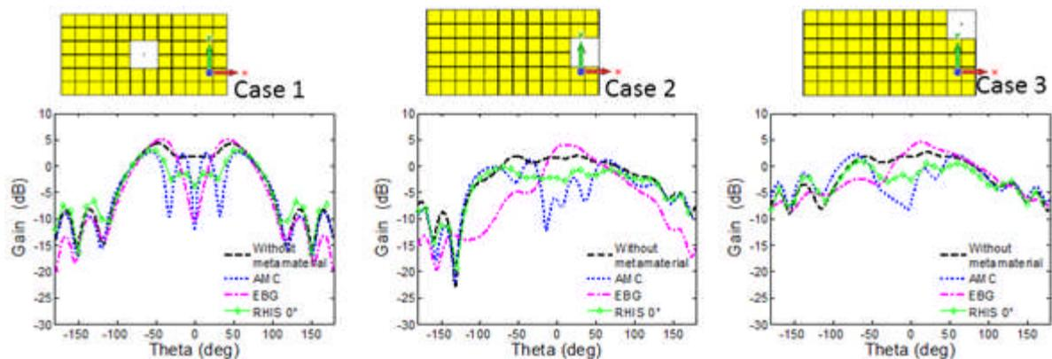
Figure 72 Gain Radiation pattern. Plane  $\phi = 9^\circ$ . Case 1: antenna at centre. Case 2: antenna at middle of the edge. Case 3: antenna on the corner
