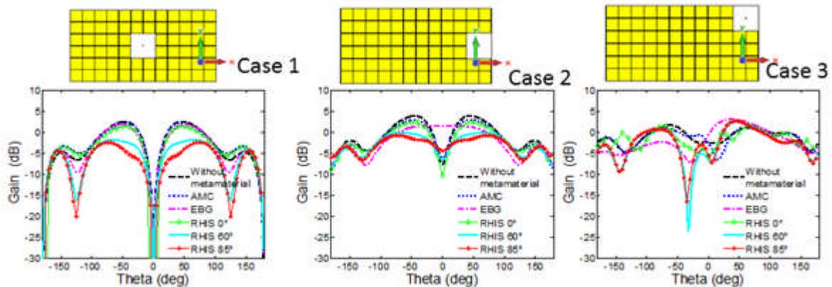
Figure 66 Gain Radiation pattern. Plane  $\phi = 90^\circ$ . Case 1: antenna at centre. Case 2: antenna at middle of the edge. Case 3: antenna on the corner
