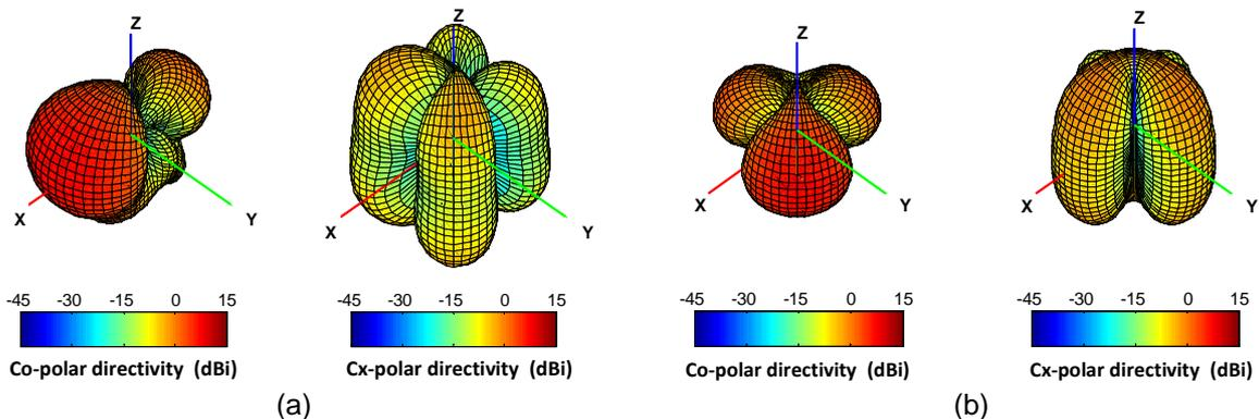
**Figure 17 Directivity pattern (Co-polar and Cx-polar components) of the circular array calculated at 1.75 GHz. 3D theoretical results (a) for the end-fire and (b) 45°-steered configurations.**
