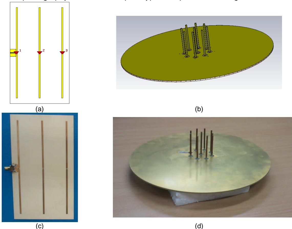
**Figure 15** Realized prototypes. Schematic view of the (a) three element array and the (b) nine element array. Photography of the realized (c) three-element array and the (d) nine-element array.
