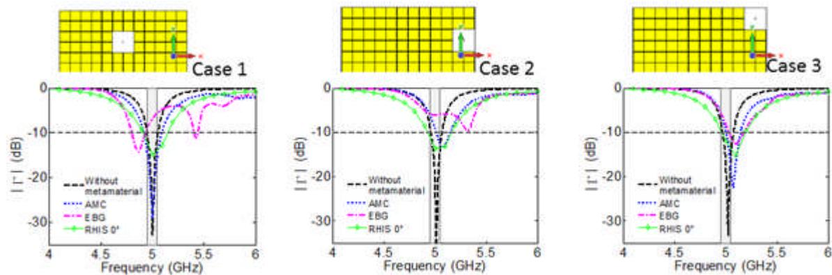
Figure 68 Impedance matching. Case 1: antenna at centre. Case 2: antenna at middle of the edge. Case 3: antenna on the corner
