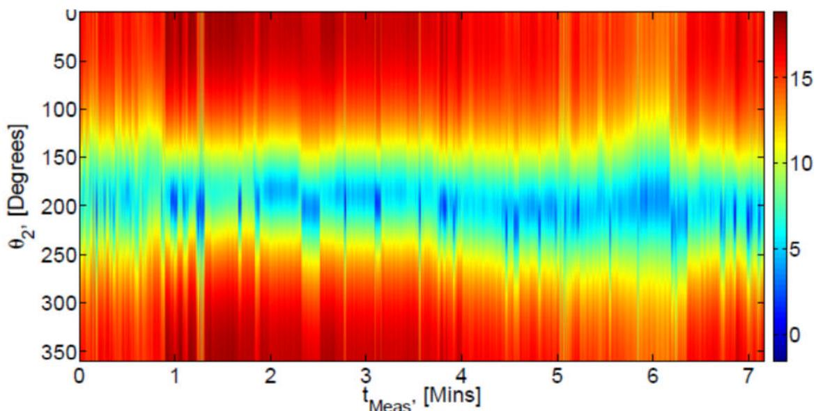
**Figure 9: Receive power in dBm over time,  $t_{Meas}$ , as measured at probes as function of angle between transmit samples:  $\theta_2$ , for the channel laptop-probes**
