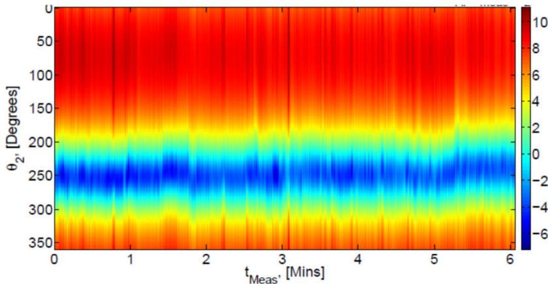
**Figure 10: Receive power in dBm over time,  $t_{Meas}$ , as measured at probes as function of angle between transmit samples:  $\theta_2$ , for the channel laptop-access point.**
