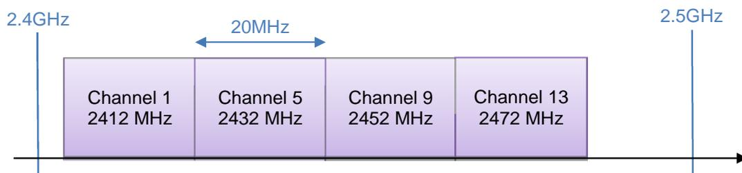
Figure 35 IEEE 802.11n adjacent channels in the 2.4GHz ISM band
