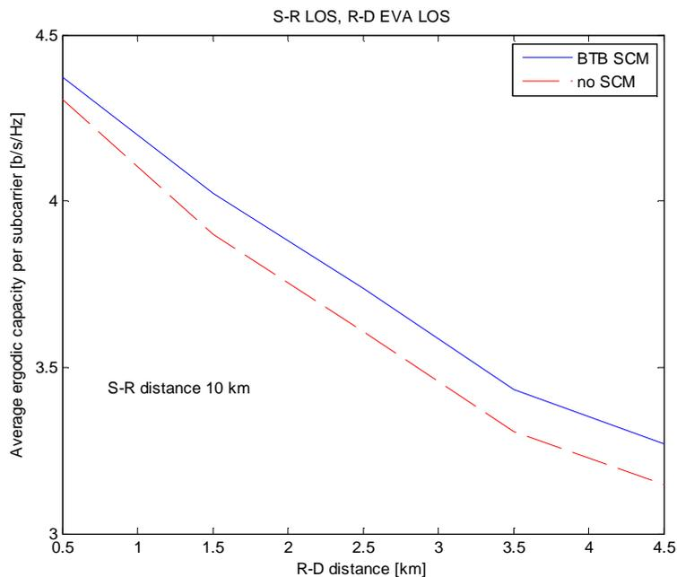
Figure 52 Average ergodic capacity per subcarrier for OFDM DF systems with BTB SCM and no SCM (S-R LOS, R-D EVA LOS scenario)
