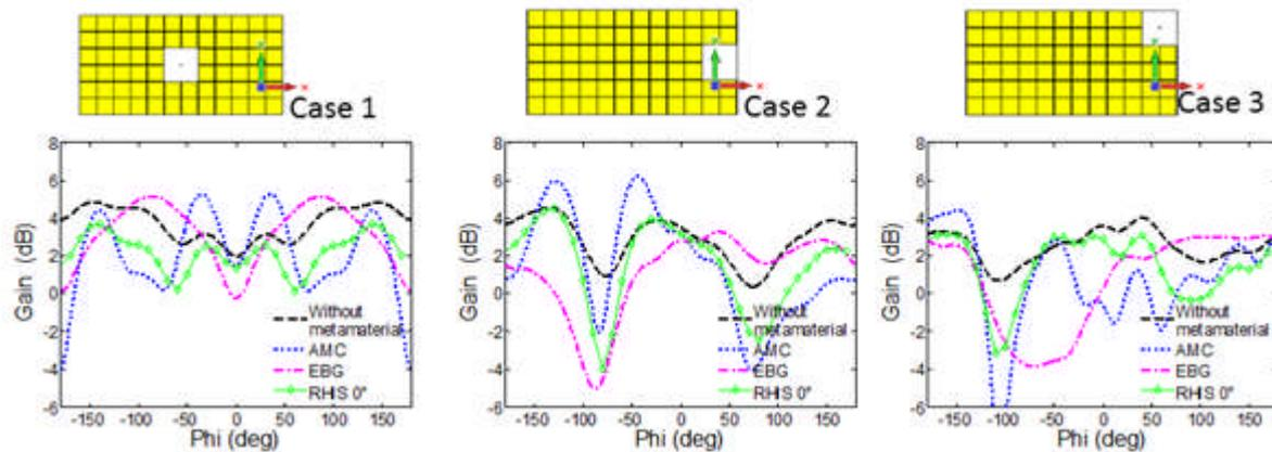
**Figure 73 Gain Radiation pattern. Plane theta = 45°. Case: Antenna at centre. Case 2: Antenna at middle of the edge. Case 3: Antenna on the corner**
