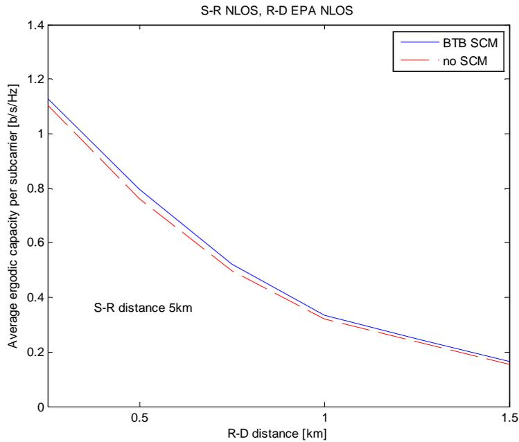
Figure 51 Average ergodic capacity per subcarrier for OFDM DF systems with BTB SCM and no SCM (S-R NLOS, R-D EPA NLOS scenario)
