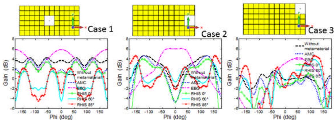
Figure 67 Gain Radiation pattern. Plane  $\theta = 45^\circ$ . Case 1: antenna at centre. Case 2: antenna at middle of the edge. Case 3: antenna on the corner
