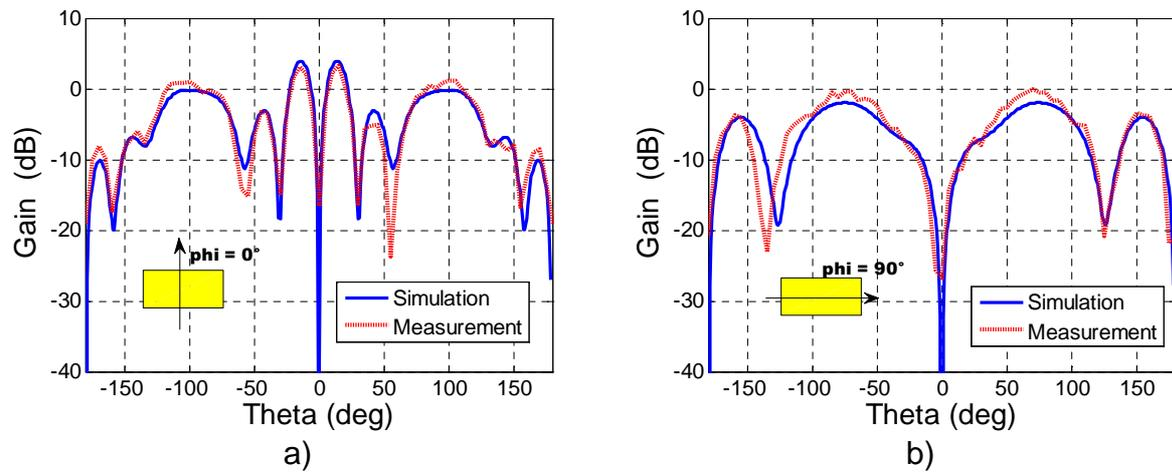
Figure 79 Gain, monopole antenna with RHIS. a) Plan  $\phi = 0^\circ$ . b) Plan  $\phi = 90^\circ$ .
