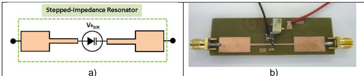
**Figure 27 a) Block diagram of the varactor-tunable SIR and b) Manufactured varactor-tunable SIR**
