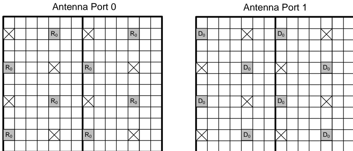
Figure 41: Antenna Port 1 configured for DMRS in the 2 CRS ports case
