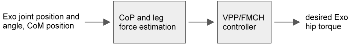
Figure 4 Structure of the VPP based controller implementation on exoskeleton
