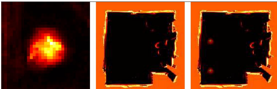
Figure 17: The occupancy map is generated from combining the human model and the background model. For each set of locations of persons, i.e. a particle, an occupancy map is estimated. Left: Human model. Middle: Background model. Right: Occupancy Map given the hypothetical location of persons (green crosses)
