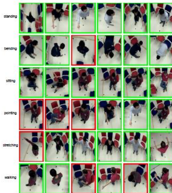
Fig. 5. Results of the posture recognition based on our top-view dataset. The example images are randomly sampled from the testing results. The text on the left indicates the ground-truth posture label of the images in the row. Postures that are correctly recognized are in green rectangles, and postures that are incorrectly recognized are in red rectangles.
