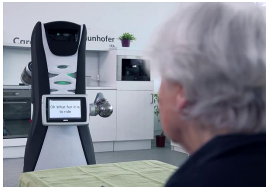
Figure 15. The new tray kinematics employed for vertically displaying the screen.
