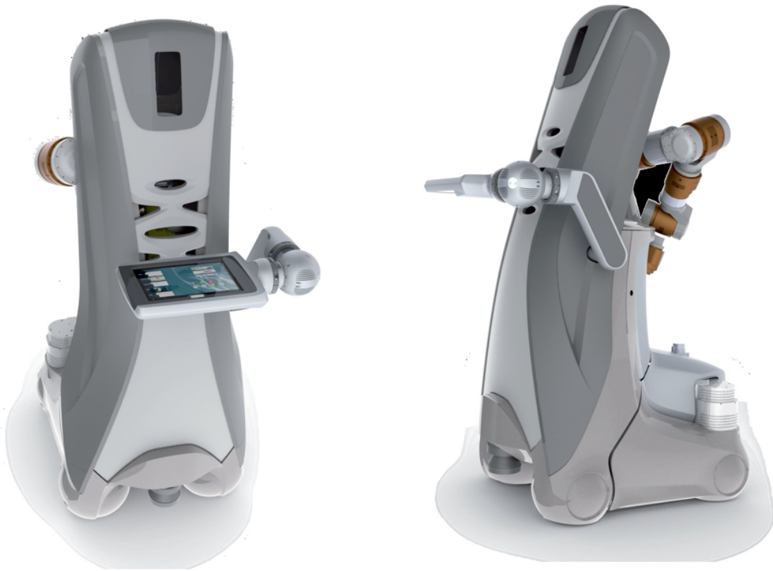
FIGURE 20. Design Drawings of the new tray kinematics with 3 degrees of freedom that allows height adjustment of the tray and switching between tablet pc and object placement
