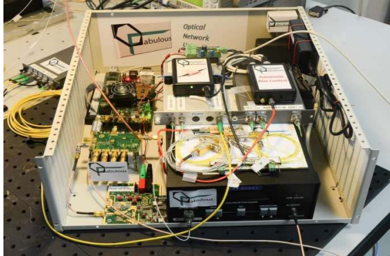
Figure 12: the real-time operating ONU, with discrete optical components and FPGA boards.
