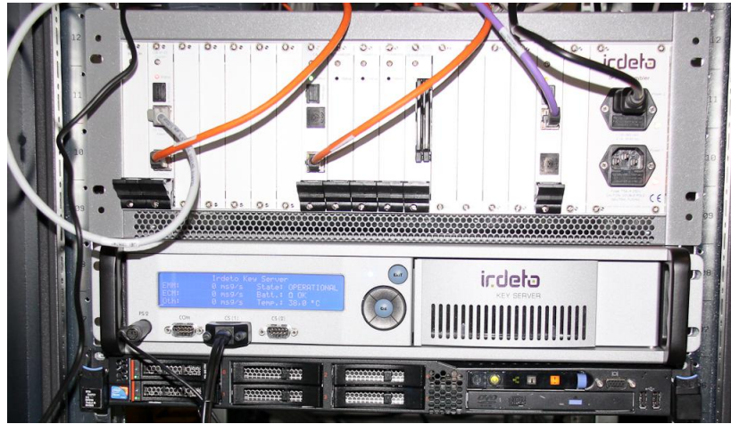
Figure 21: Encryption components: IRD IPTV Scrambler, IRD KeyServer, and IRD KMS.
