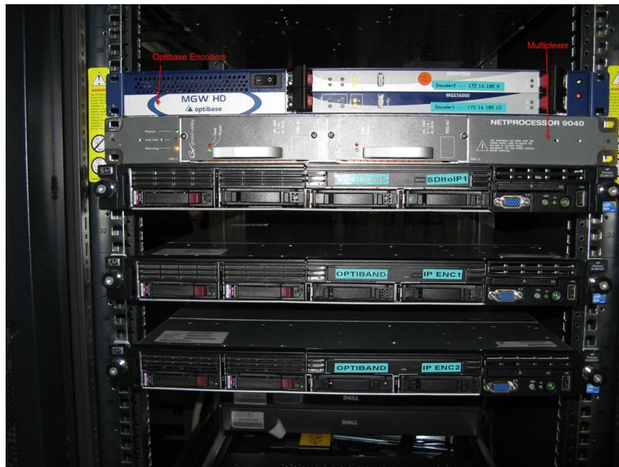
Figure 3: Live Encoders - The equipment are listed on the right side of the picture
