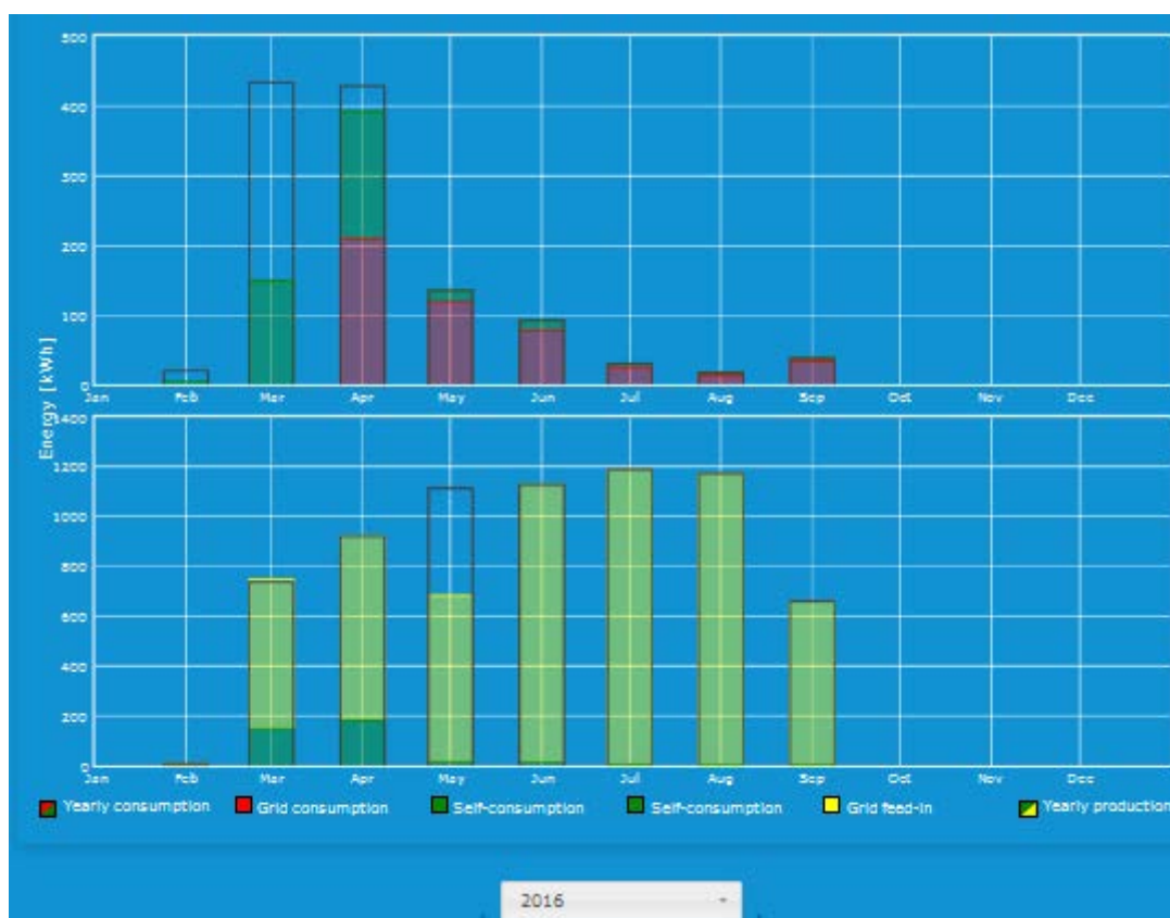
Figure 34: PV energy yield in green (light green shows the feed into public grid and the dark green the self consumption amount) and the consumption from the grid (red).
