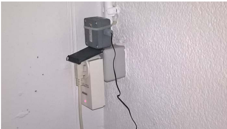
Figure 23: Smart plug as plugged into the socket to measure the consumption of the freezer and the radio transmitter of the T-sensor inside the freezer on top of the socket.
