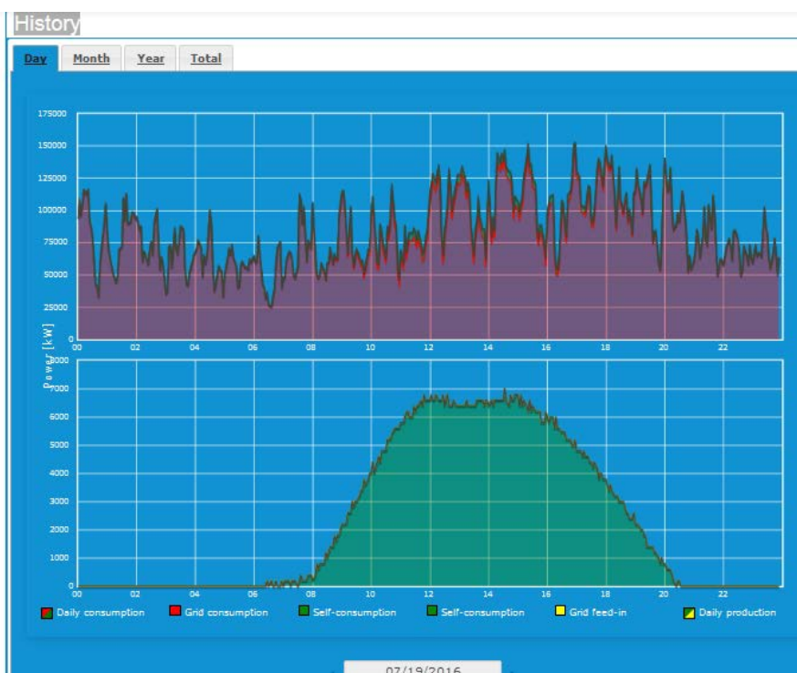
Figure 4: Top shows the power consumption and bottom the power yield of the PV system. The power yield curve vs. time shows often a drop-shift regularly at the sun's climax at very sunny days probably due to regulation of the inverter to 70% of W_{p_{max}} .
