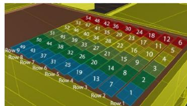
(d) The composition of the PV/2 system on the facade.
