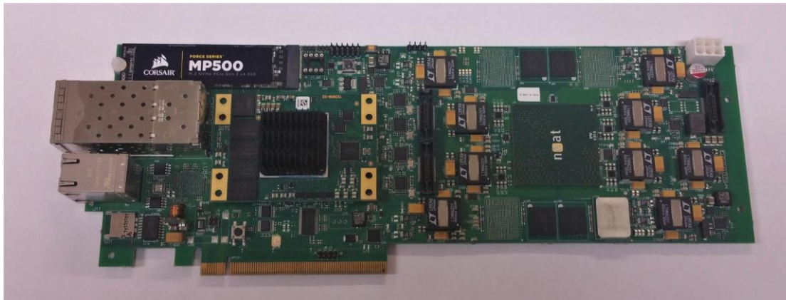
4: The EUROSERVER designed, NEAT produced, prototype board. Not shown are a Trenz 0808 module and a SIP
