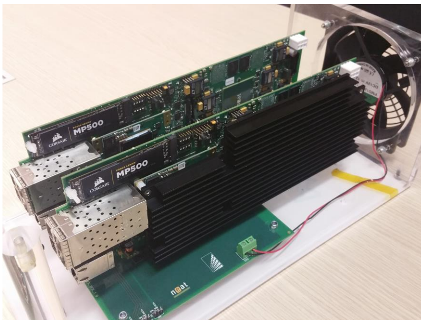
Figure 9: A pair of EUROSERVER boards, assembled onto a backplane with electrical connectivity, designed by EUROSERVER and produced by NEAT
