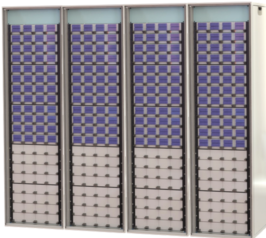
Figure 7-9 Illustration of the physical size required for a 12,288 port single-sided optical switch fabric using a 3-stage folded-Clos architecture
