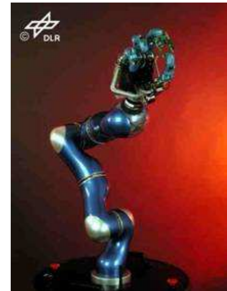
DLR lightweight arm Payload/mass ratio = 1
