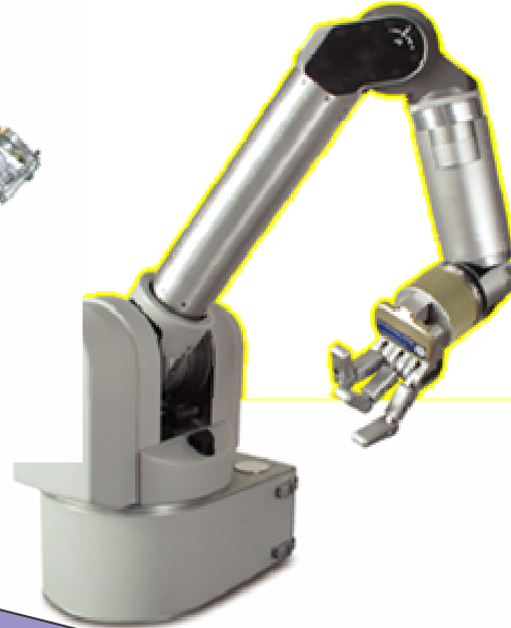
WAM arm (Barrett Technologies) High speed: 20 m/s
