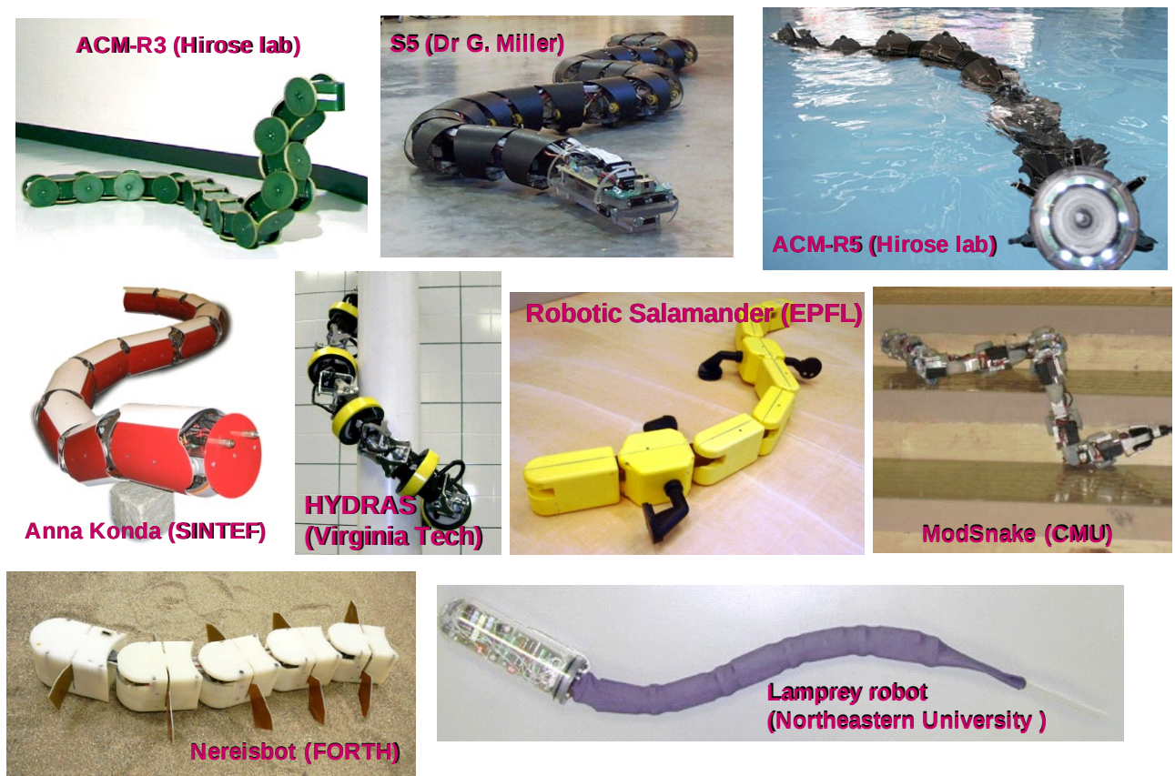
Figure 2: Hyper-redundant robotic locomotion systems.
