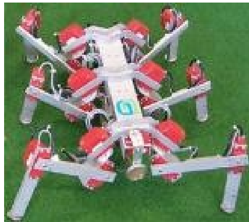
Figure 4.10 Tarry the Hexapod to demonstrate Walknet
