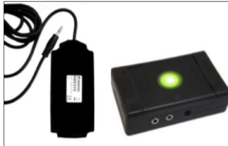
Figure 10. Bed presence sensor (left) and concentrator (right).
