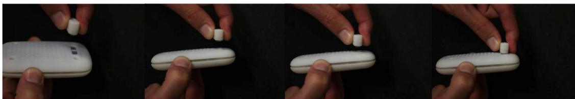
Figure 54. Charging sequence for the fall detector.
