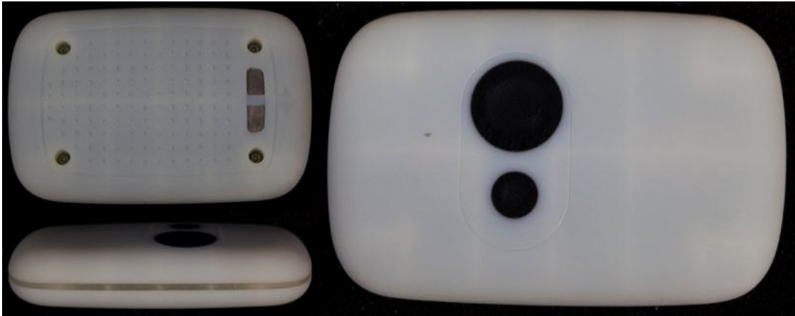
Figure 4. Case of the fall detector.
