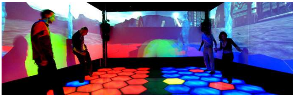
Fig. 11 - An application using the pressure sensitive floor in the XIM
