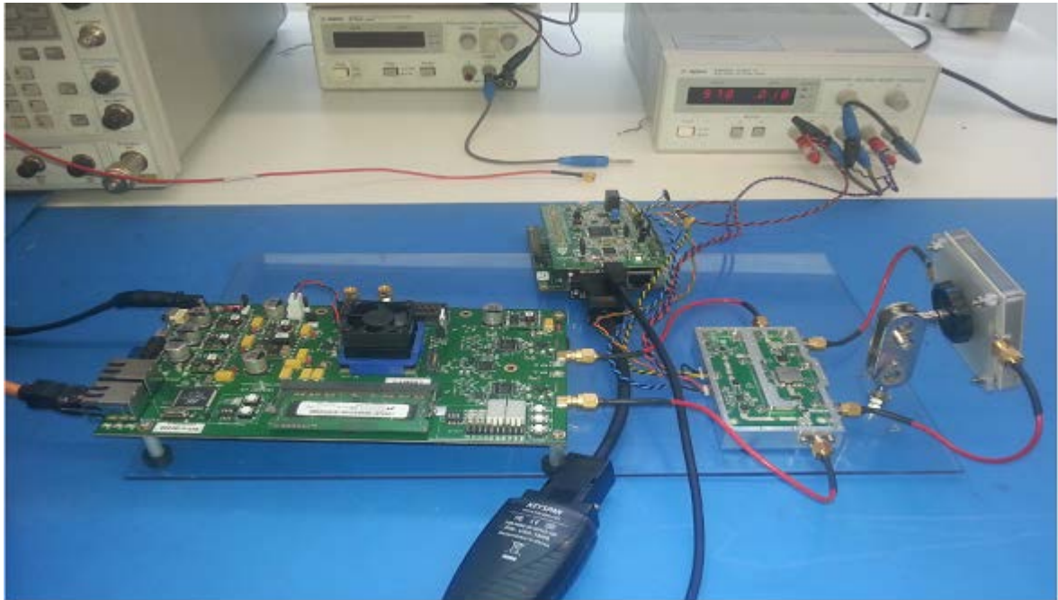
FIGURE 46. Picture of the dual-port antenna experimental setup including WARPv3, active cancellation network and dual-polarized antenna.
