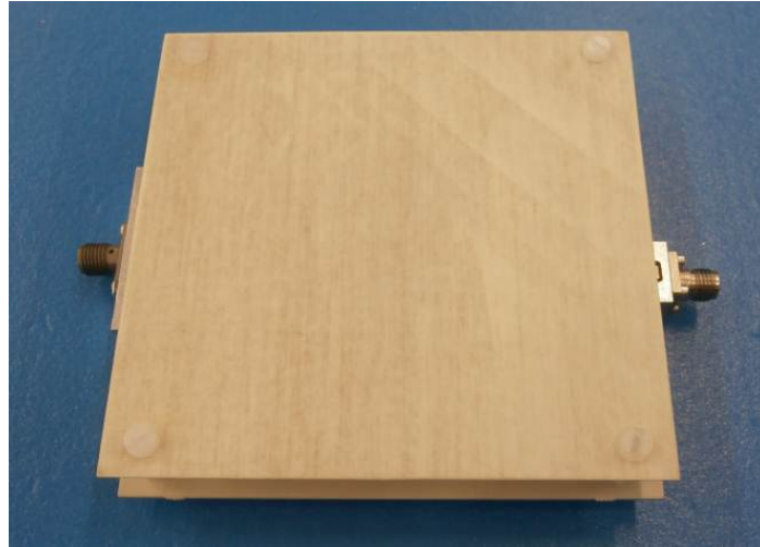
FIGURE 3. Final dual-polarized antenna with SMA connectors.
