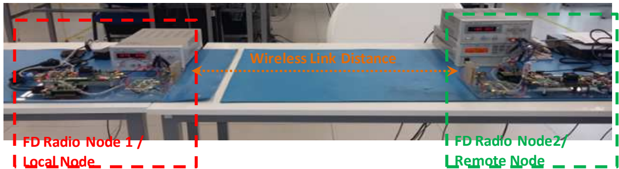
FIGURE 53. Picture of the evaluation setup with the dual-port antenna radio node.
