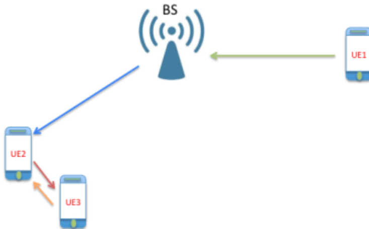
Figure 12. A LTE small cell with a BS and full-duplex device-to-device UEs.
