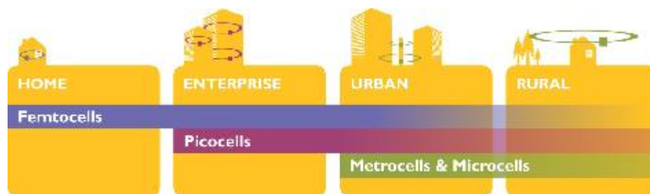
Figure 5. Small cell technologies and their typical operation environments [34].
