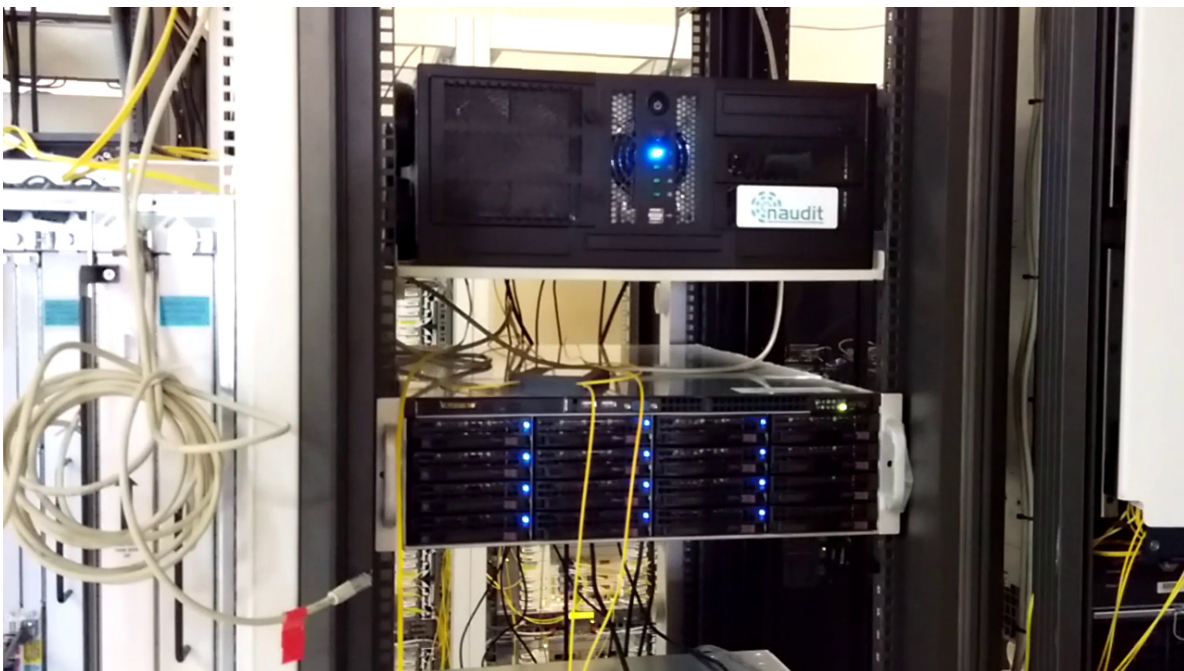
Figure 61: Picture of the traffic generator and the monitoring probe in the testbed
