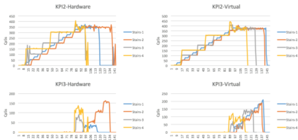
Figure 50 – KPI 2 and KPI 3 results of a MGW running on a virtualized vs HW-based environment
