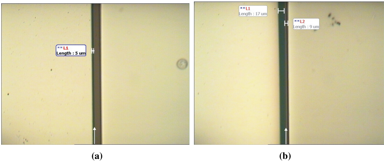
Figure 2.5.3. Optical microscope images of devices fabricated using a thick SU-8 25 layer as integrated shadow mask. The distance between the metallic layer (white area) and the insulator edge, indicated by the white arrow, is 5 \mu\text{m} and 17 \mu\text{m} respectively for (a) and (b).
