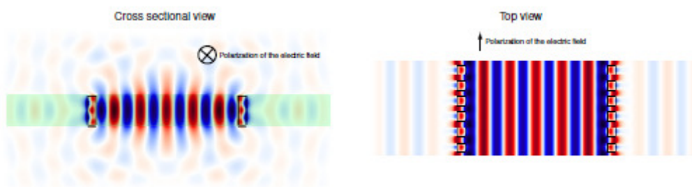
Figure 2.2.12. Ab-initio calculations (3D finite-difference time-domain method) of a Fabry-Perot cavity implementing the hybrid concept. The electric field in the direction of the shown arrow (= polarization of the source which excites the cavity) is plotted. The silicon blocks are shown as black lines. The green area in the cross sectional view denotes the organic layer.
