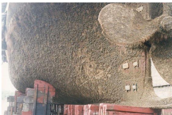
Ship hull fouled by barnacles (Akzo-Nobel)
