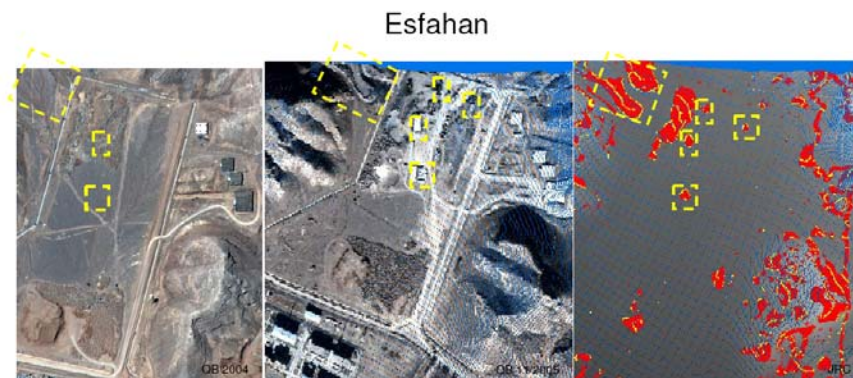
3D Change detection (right) using QuickBird stereo pairs of June/July 2004 (left) and November 2005 (middle), Esfahan © JRC
