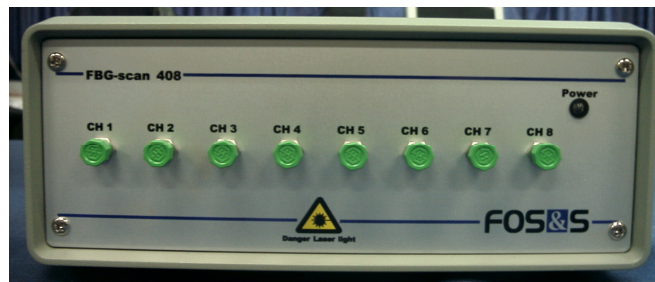
Figure 12: Photo of the front panel of the interrogator prototype
