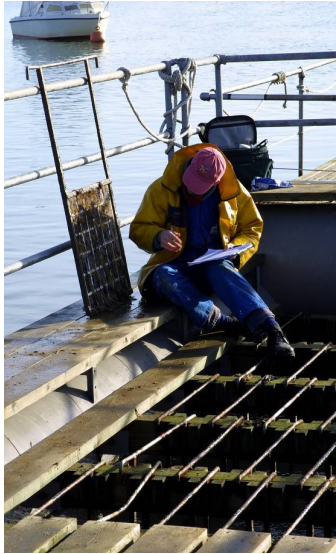
Panel testing from rafts (AKZO)
