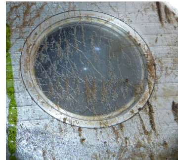
Above: top image shows fouling of optical window after 5 weeks immersion. Bottom image shows reduced fouling of optical window coated with TEER's SiOx-like coating, after 7 weeks immersion
