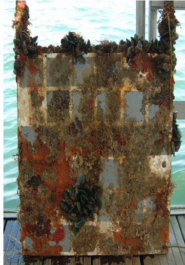
Panel testing from rafts (AKZO)
