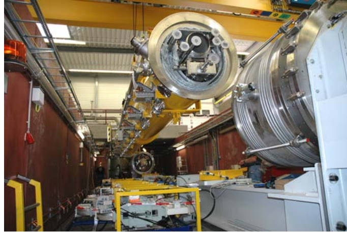
Figure 9: Installation of a 12 m long cryomodule in the CryoModule Test Bench (CMTB) at DESY.
