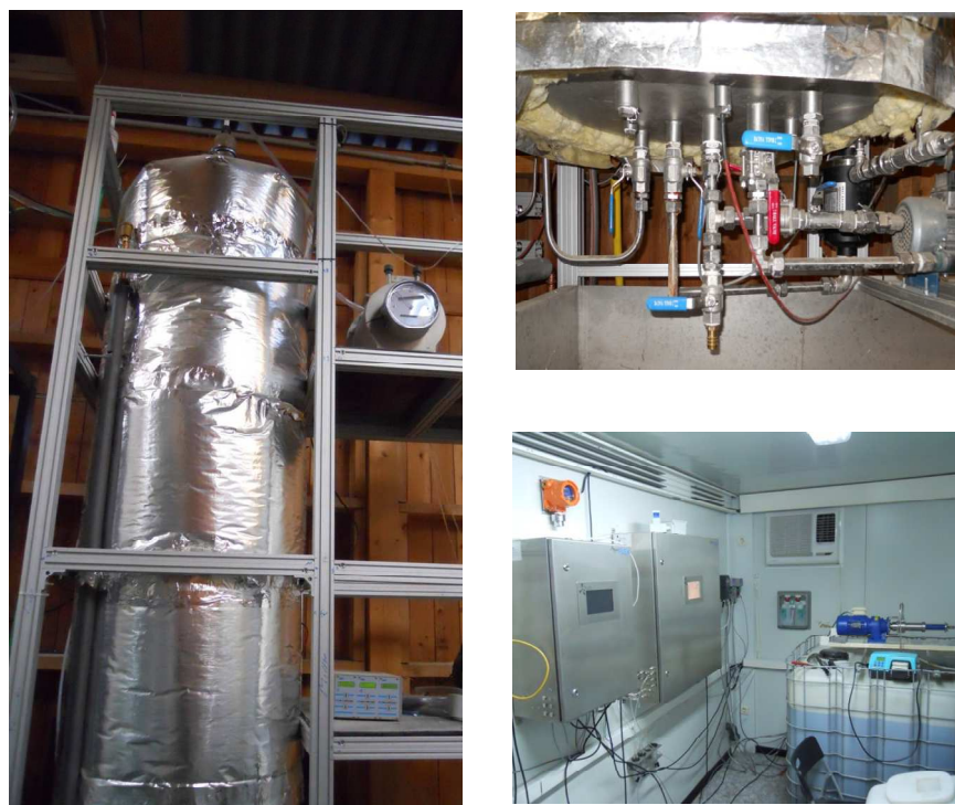
Figure 8: 600 L combined fluidized and trickling bed (CFTB) reactor; A. Bioreactor system after installation with glass wool insulation; B. Installations and connections at the bottom part of the bioreactor; C. Gas analysis system and control system and at the right side the molasses container.
