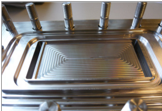
Figure 18 Feed compartment of the high pressure membrane module.
