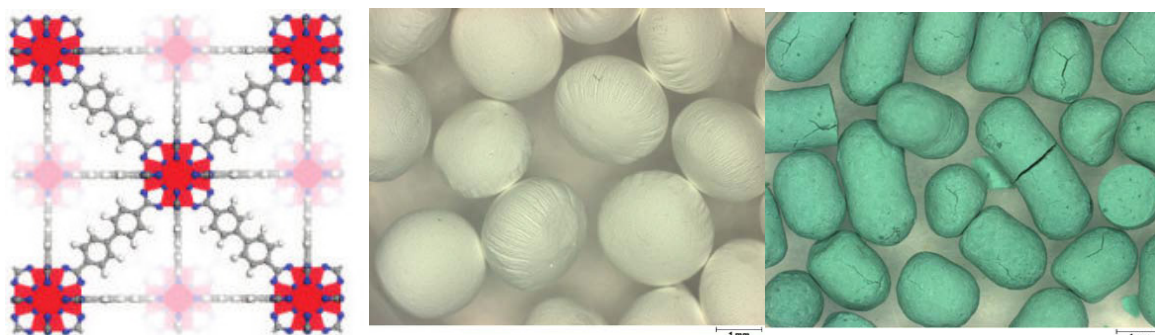
Figure 15 From left to right: Ball-stick model of one of the MOFs studied (UiO-67). Formulated MCM-41 spheres made by the alginate method (middle). Formulated particles of a MOF (USO-2-Ni) made by extrusion method.
