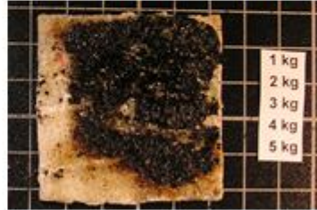
SCRATCH ADHESION TEST
