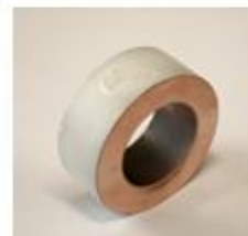
Airbrush/Cu (sand blasted)/ZrO 2 /Silicone/ 200° C/1h/Air/ ca. 200µm
