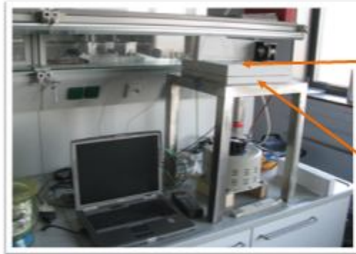
Experimental set-up for measuring the thermal barrier effect
