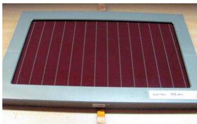
Figure 5.3 A double glass-substrate single cell from 3GSolar.
