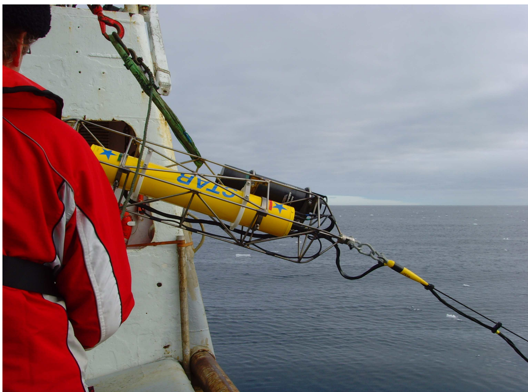
Figure 8. Deployment of the STAR system for recording data from the hydrophone arrays
